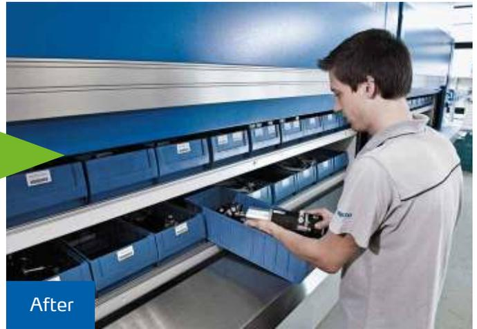
Automated storage and retrieval systems deliver stored items to the operator; eliminating workers climbing, bending, reaching, twisting and lifting activities commonly associated with shelving. For heavy inventory, ergonomic hoists, lifts, carts & transport tables can be easily integrated into the workstation. This OSHA friendly work environment reduces worker fatigue and risk of worker injury.
