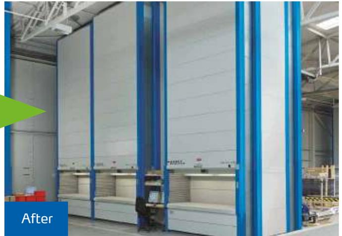
When compared to standard shelving, automated storage and retrieval systems can save up to 85% floor space. Eliminating aisle space required for shelving and utilizing the complete floor to ceiling height provides organizations with a smaller footprint.
