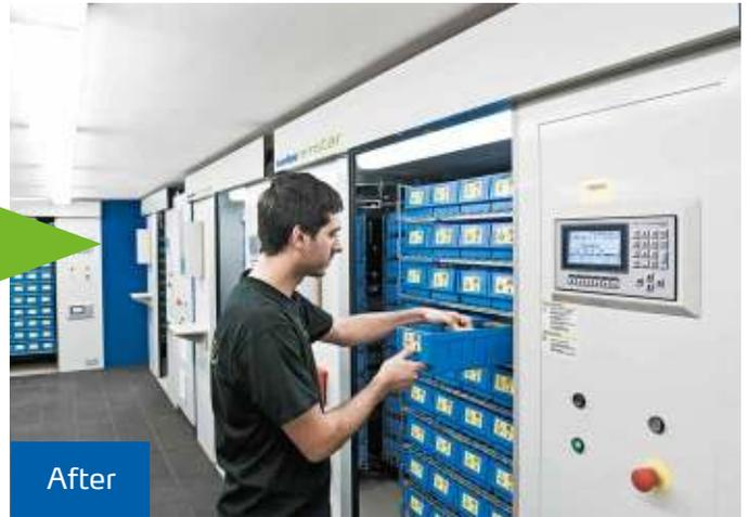
Automated storage and retrieval systems allow operators to perform at higher levels. By delivering items directly to the operator, travel and search time commonly associated with shelving is drastically reduced. This allows the operator to spend more time picking, increasing overall productivity.
